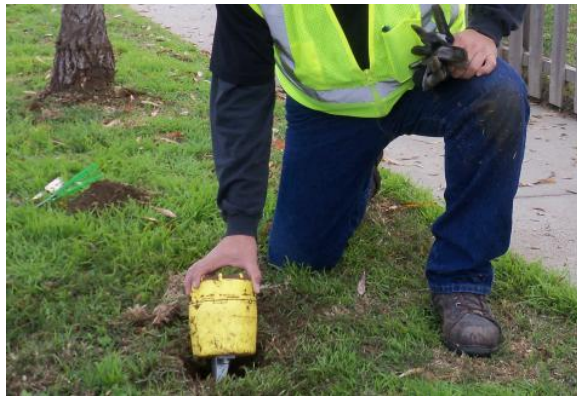
Geophones (nodes) are small, electronic receivers designed to pick up seismic vibrations below the earth's surface.
