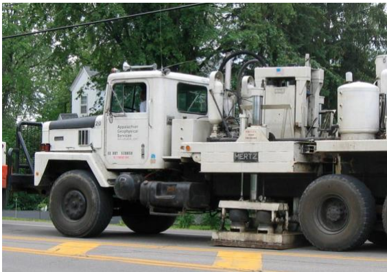
Vibroseis truck used for seismic testing on Warren Road in Ithaca, 2007.
